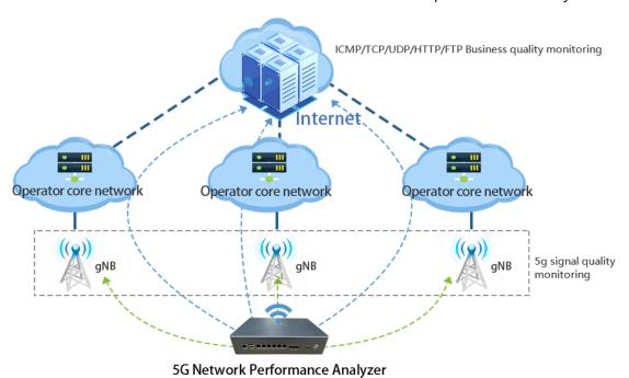
The V1500 APMVista 5G Network Performance Analyzer can obtain 5G wireless signal quality by connecting to a 5G base station. The indicators that 5G wireless signal monitoring can collect include:
