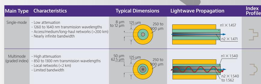
**Refractive index:** A measure of the speed of light in a material. The n1 and n2 are the respective refractive index of the cladding and the core. n1<n2 is the condition for the light to travel down the fiber. *Index profile:* Variations of the refractive index along a fiber diameter.
