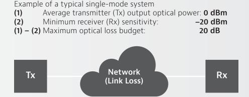
Optical loss budget must consider both link loss and system power margins to allow for the effects of environment, aging, and eventual repairs.
