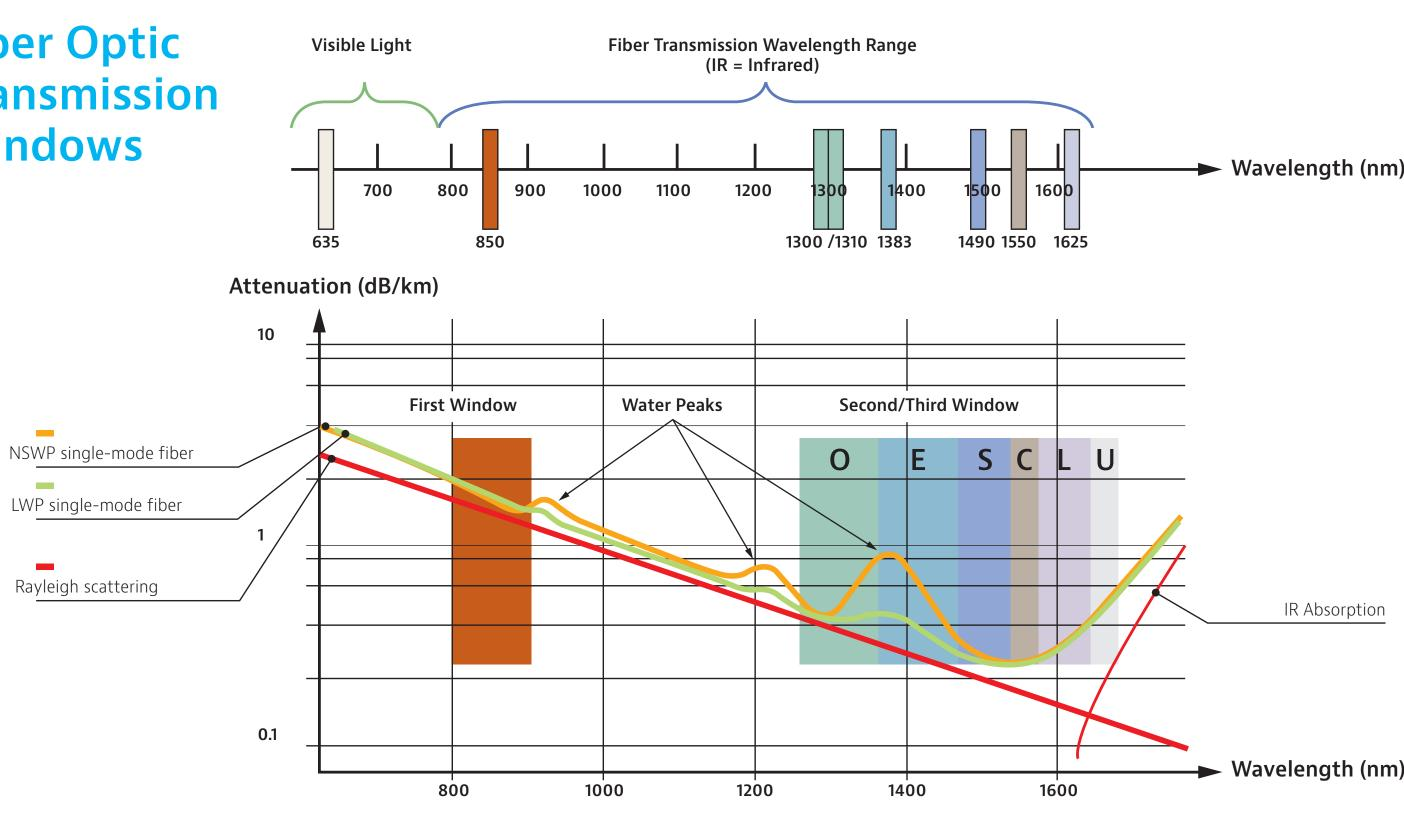
Attenuation results from various scattering and absorption mechanisms and is wavelength-dependent.
